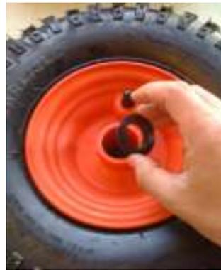
**Step 2:** Use a Rubber Mallet to fasten in the wheel retainer ring (P14)
