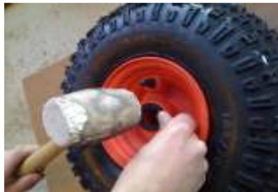
**Step 3:** Drop in your wheel bearing (W-RB 60) and repeat steps 1 and 2 to fasten in the wheel bearing (W-RB 60)
